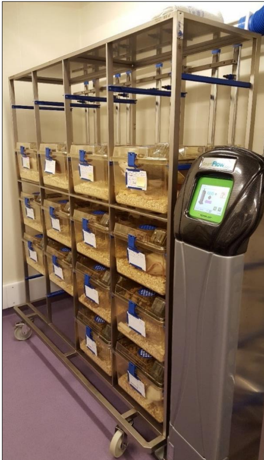
Figure 5 IVC rack with automated air supply from the integrated ventilator system in the animal facility.
