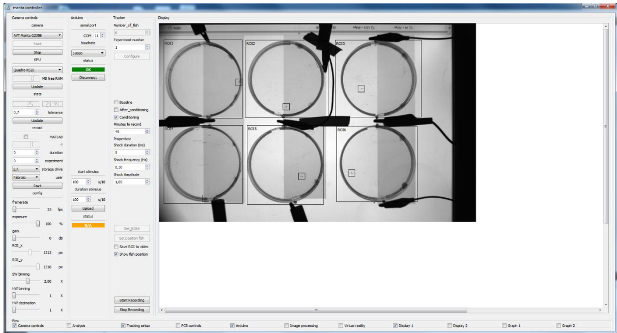
Figure 15) Software interface during conditioning of six zebrafish in a round shape arena. The six region of interest (ROI) are highlighted on the live image detected from the camera and the fish position is on-line plotted as a square box over the fish.
