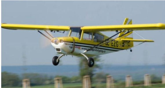
Figure 3.8: Bellanca Super Decathlon XXL UAV used for experimetal verification.
