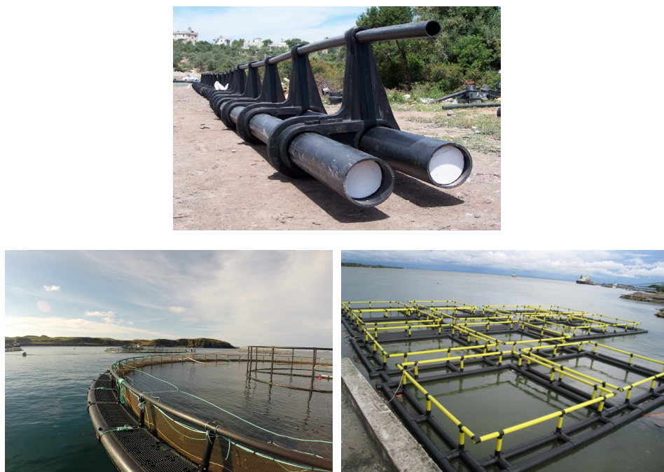
Figure 1.5: Details of HDPE floaters. The straight pipes in the upper photo (FAO) are forced into circles and squares and welded together to become the floaters in the lower photos ( www.worldfishing.net ).
