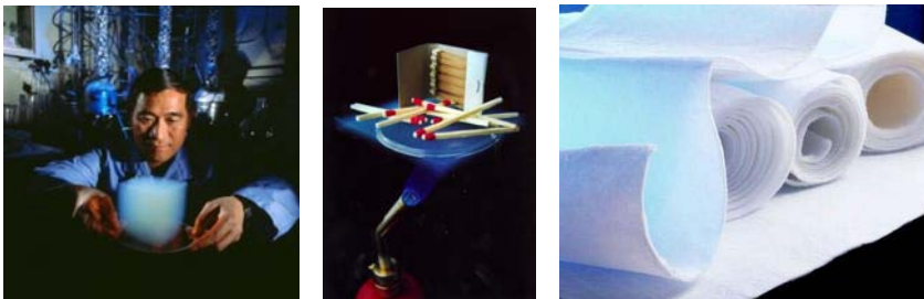
Figure 5. (left) Peter Tsou from NASA with a translucent aerogel sample developed for space missions (NASA 2010), (middle) matches on top of aerogel are protected from the flame underneath (NASA 2010) and (right) an example of aerogel as a high performance thermal insulation material (Aspen Aerogels 2009).
