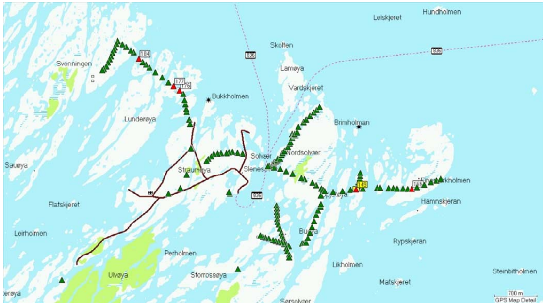
Figure 8. Power lines and poles inspected on Solvæøyene on Lurøy in July 2008.
