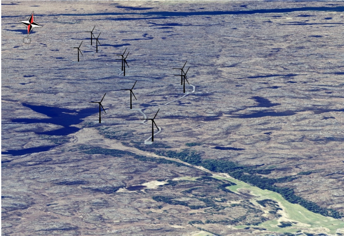
Figure 38. Example of aerial image draped on to our new DEM. Elevation is exaggerated to give a better visual impression of the topography. Wind turbine number 21 in front.
