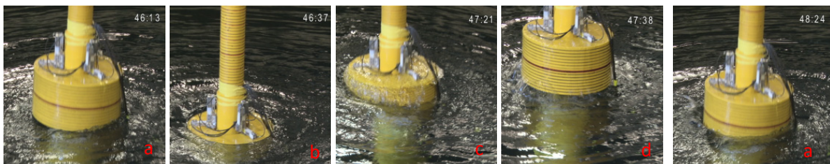
Figure 4. Strongly nonlinear phenomena in the model test for incident waves with H=9\text{m} and T=15\text{s} : water entry (a and b), green water (b and c) and water exit (c and d). Time increases from left to right.
