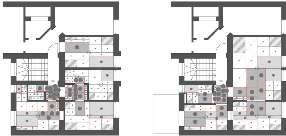
Figures 6(b) and 6(c). Placement of perceptual centers: Plans of the first floor before (6b) and after (6c) the building renovation, scale 1:200. Residential building, Cologne, Germany, © [DETAIL]. Reproduced by permission of DETAIL.
