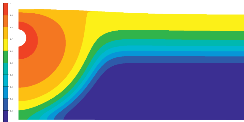
Figure 15: Frost heave: Ice saturation at the final step i.e. after 358 days.
