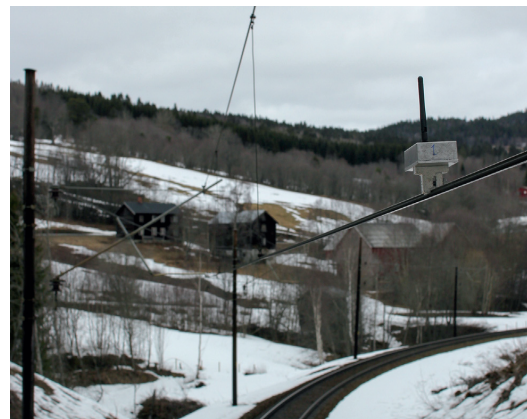
Fig. 1. Sensor mounted on the contact wire. Photo: Petter Nàvik/NTNU.
