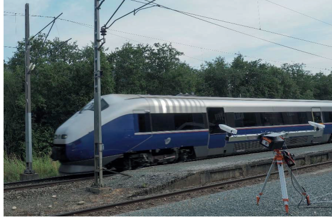
Figure 1. Camera set up for photogrammetry at Hovin. Photograph: NTNU/Petter N avik.
