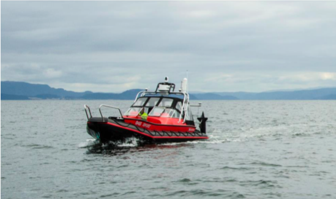
Figure 5.9: The vessel Telemetron was used as a test platform for the SB-MPC collision avoidance algorithm.
