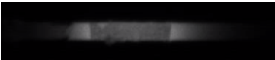
Figure 3.9: Image captured using the camera in the CO 2 set-up. The melt zone is clearly visible due to the difference in emissivity of the liquid and solid phase. The camera was placed perpendicular to the laser axis.
