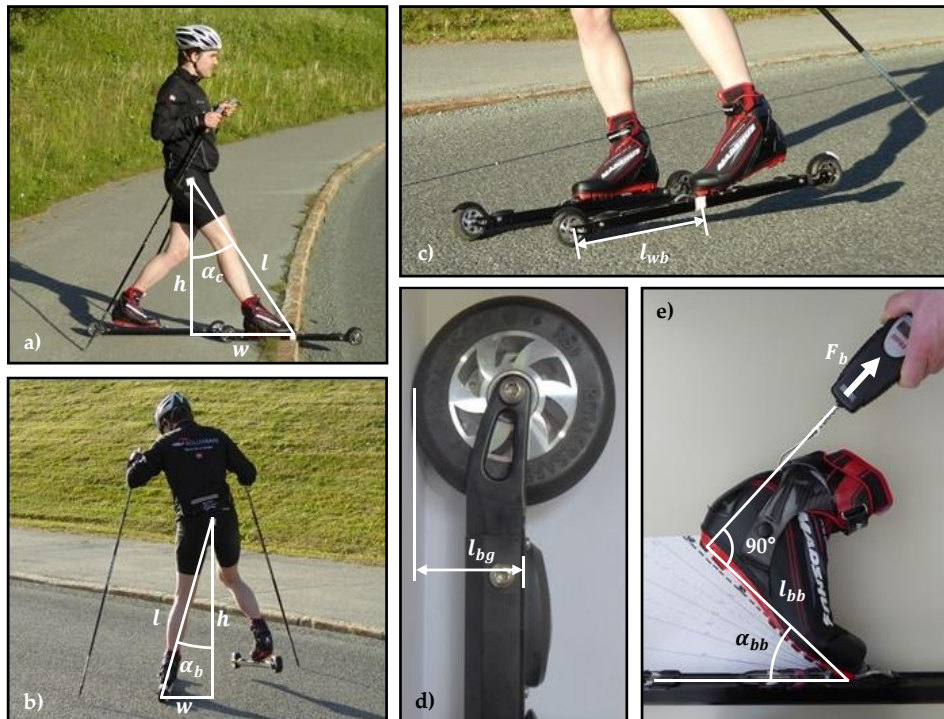
Figure A 14: Peak load events: a) Catching a curb stone performing a telemark movement, b) altering push braking, c) side view during alternating push braking, d) side view of the skating roller ski, e) measurement of the binding rubber compression torque
