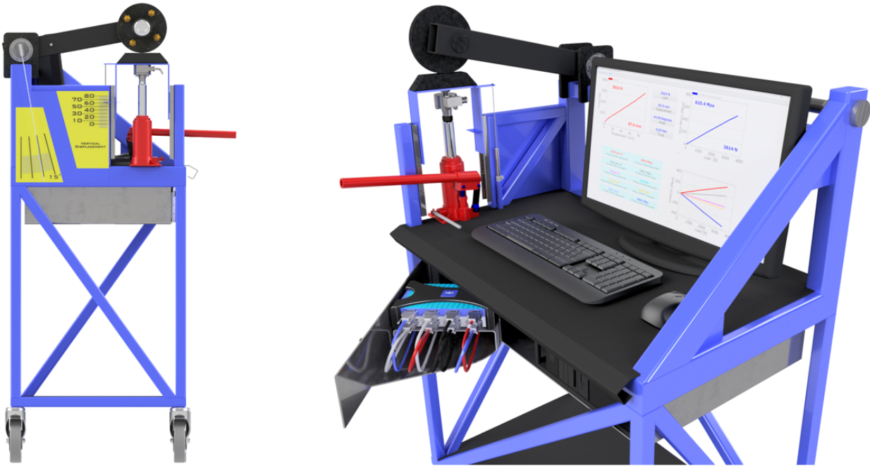
Figure 4.16: CAD of Finished Rig
