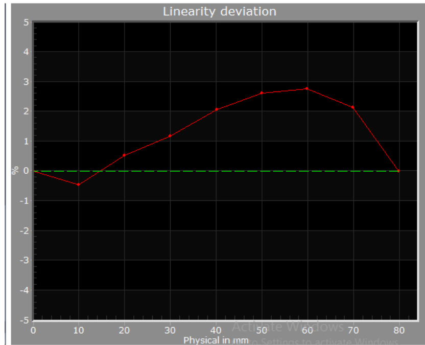
Figure 5.2: Calibration of Displacement Sensor
