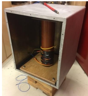
Figure 53: The Coil Installed inside the Finished Faraday Cage
