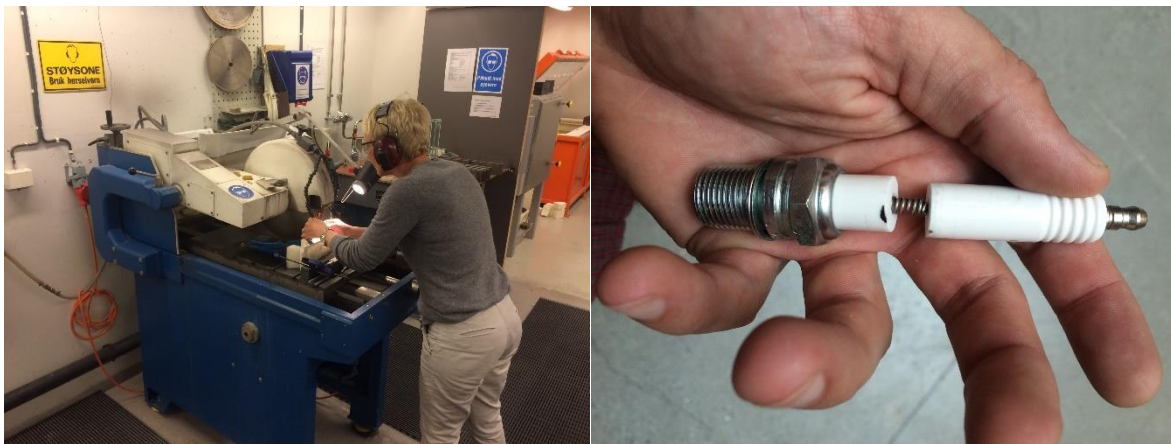
Figure 64: Removing Internal Resistance Inside the Spark Plug
