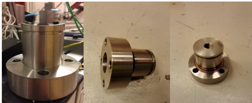
Figure 36: Final Outcome of Rig Plug for M18 Spark Plugs
