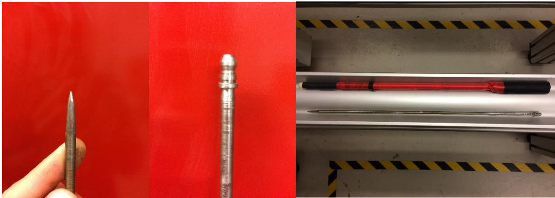
Figure 65: The 40 [cm] Machined Steel Rod with Pointy Tip and Terminal End Connector
