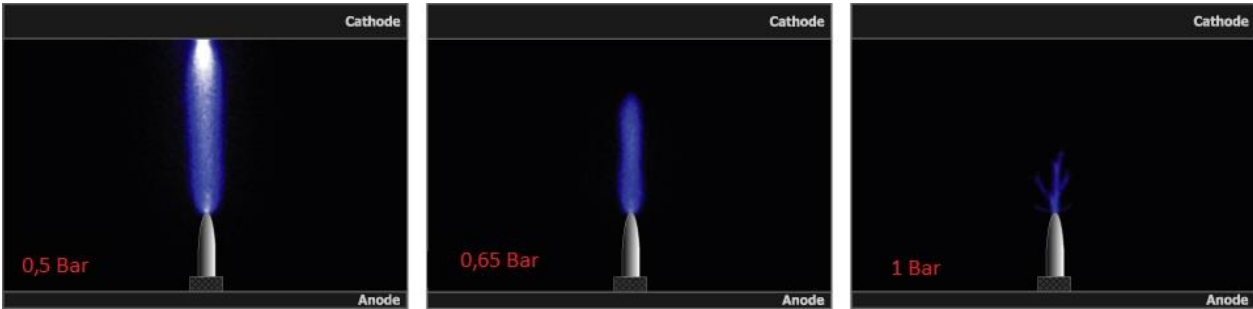
Figure 30: Corona Streamers in Different Electrical Fields Due to Pressure Variation [31].
