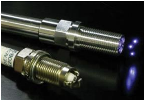
Figure 25: Laser spark design by NETL 7
