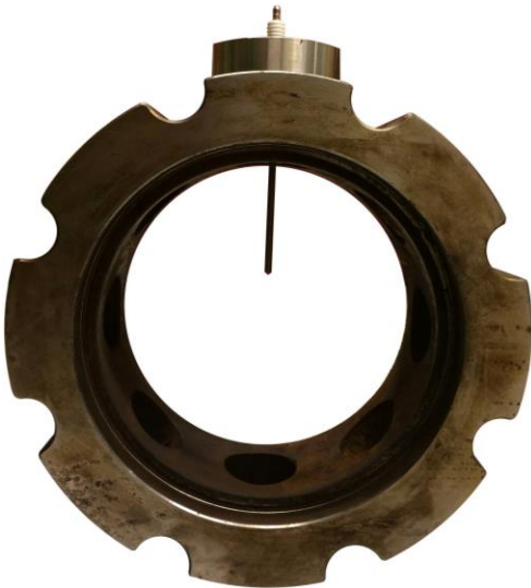
Figure 46: Position of Modified Spark Plug Tip inside the CVCC
