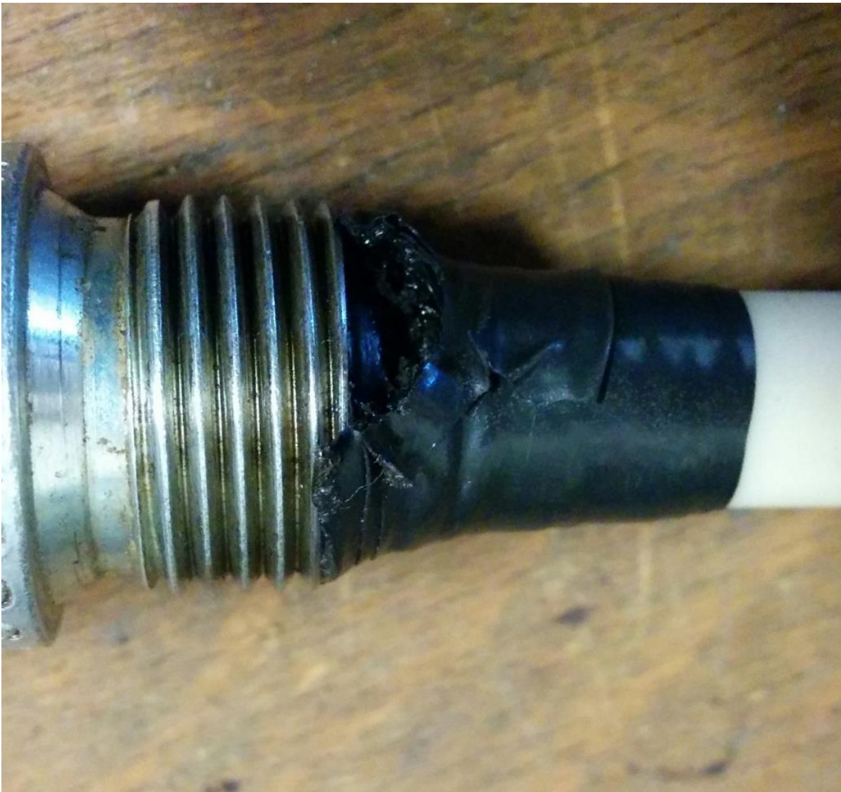
Figure 63: Detailed Picture of Scorched Insulating Tape After Test 1
