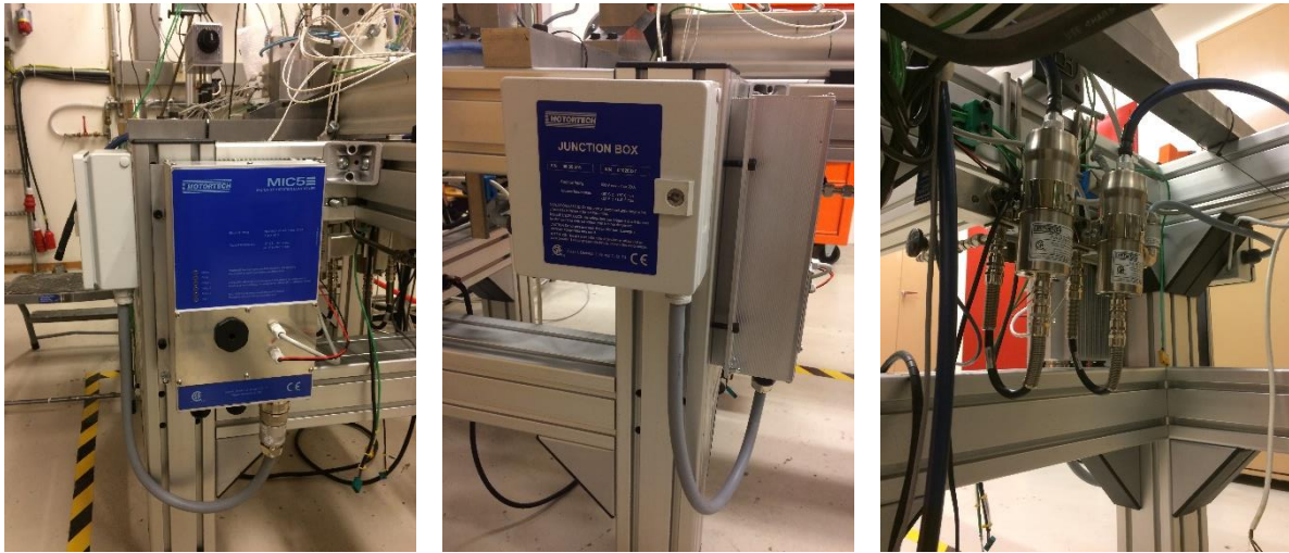
Figure 35: The Conventional Ignition System Installed on the CVCC
