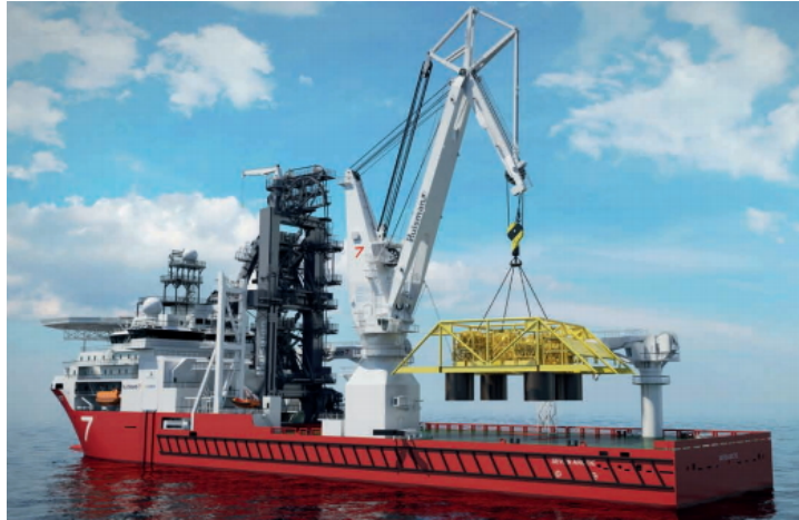
Figure 2.6: Subsea template lifted off deck (Subsea 7 2015)
