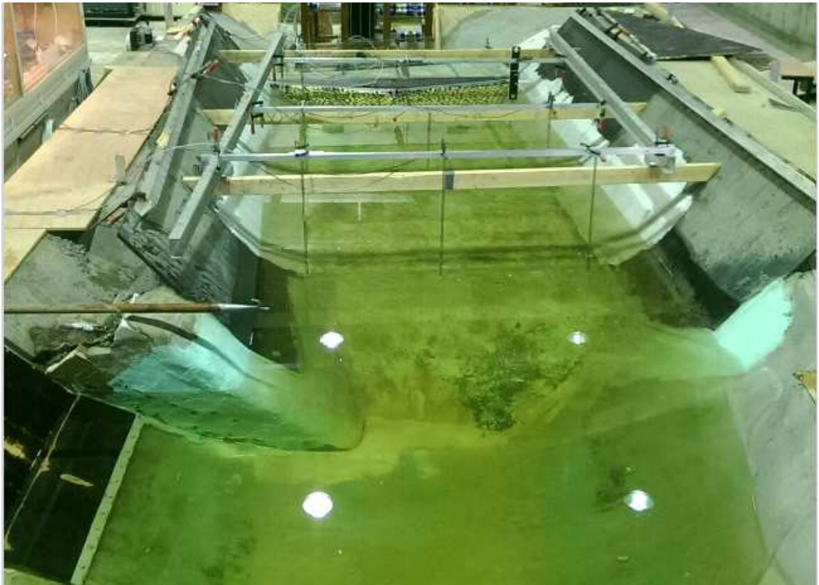
Figure 10 Photo of reservoir. The avalanche slide is just visible to the near left. Nine wave sensor partially submerged in the water, and the chevron dam in the back.
