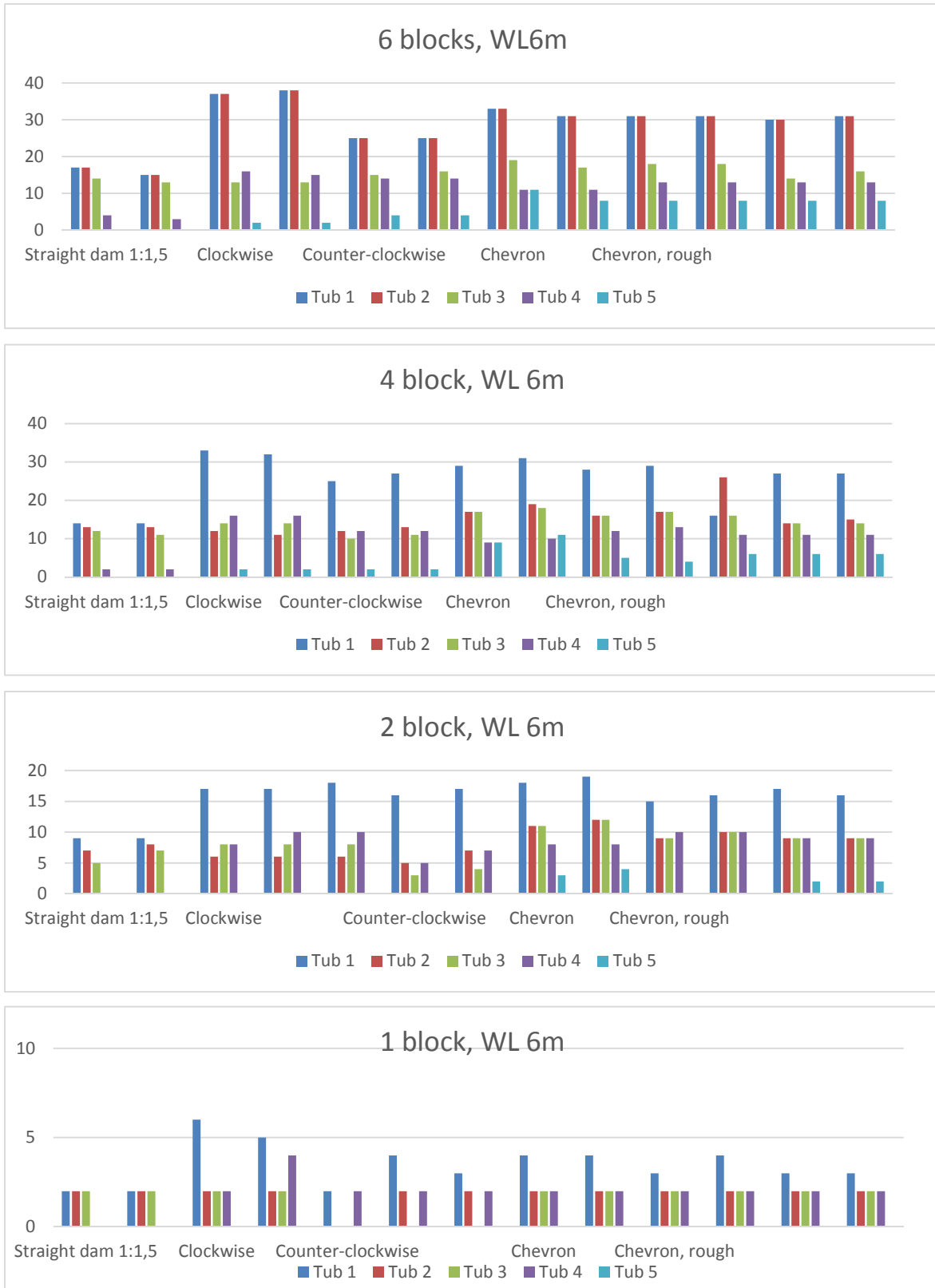
Figure 27 Graphs showing overtopping [liters] for different avalanche sizes and dam designs for LRWL
