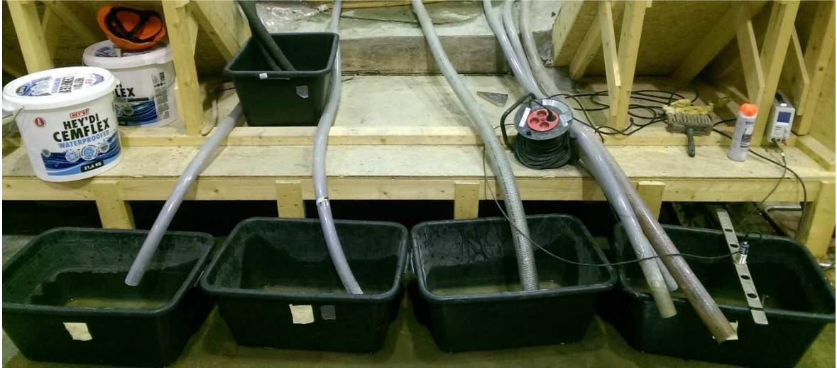
Figure 20 Overtopping tubs. The tubs has a filling curve with measured mm to liters. Measuring the water height and plotting against the filling curve gives volume of water
