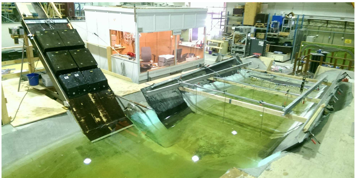
Figure 11 Model in the waterways lab. Slide to the left, wave breakers not visible at the bottom. 9 wave sensors, control room booth and not visible in the back, overtopping tubs and measuring sensors.
