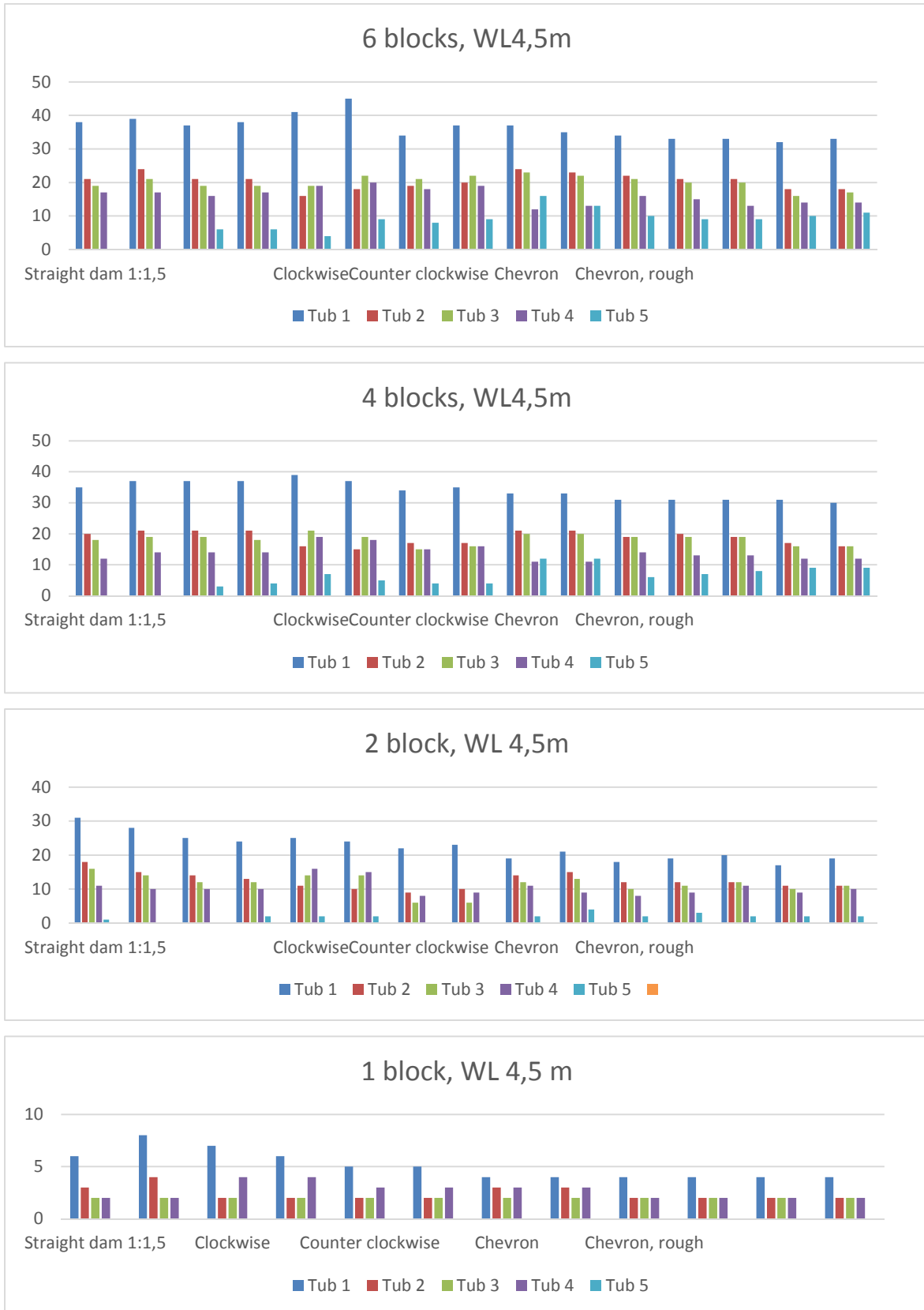
Figure 29 Graphs showing overtopping [liters] for different avalanche sizes and dam designs for HRWL
