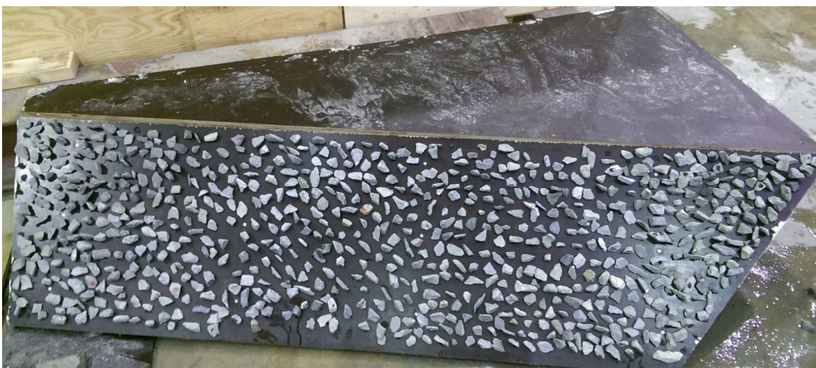
Figure 15 Dam model, rotated dam 1:1,5. It has stones on both sides so it can be rotated clockwise and counter-clockwise
