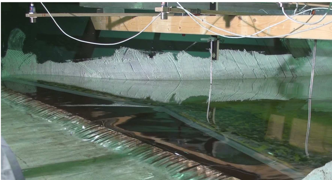
Figure 19 Dam overtopping. The ultrasonic sensors are visible top left and top middle
