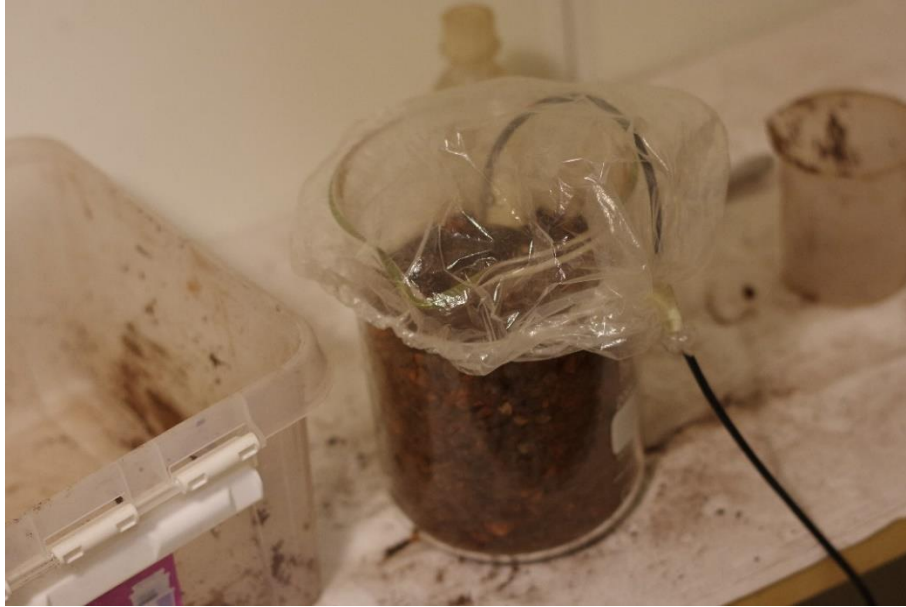
FIGURE 6.2 SOIL SPECIFIC CALIBRATION. 1.5 LITER OF SOIL INSIDE A BEAKER GLASS OF 2 LITER
