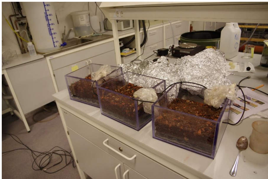
FIGURE 6.5 FROM THE FIRST ATTEMPT AT FIELD SPECIFIC CALIBRATION WITH SUBSTRATE S2, DRAINAGE ELEMENT IS INCLUDE
