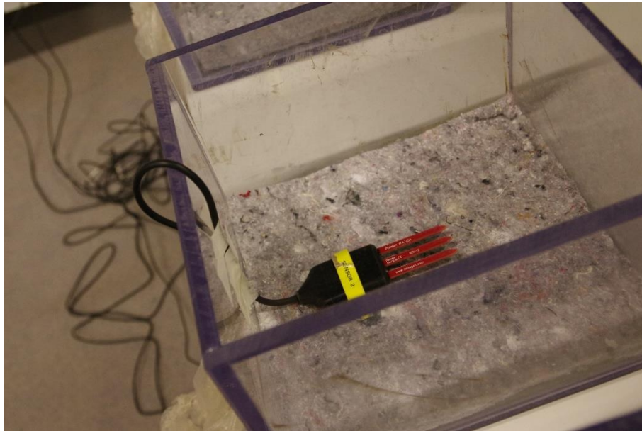
FIGURE 6.3 AN ILLUSTRATION OF HOW THE SENSOR WERE MOUNTED DURING THE EXPERIMENT WITH FELT
