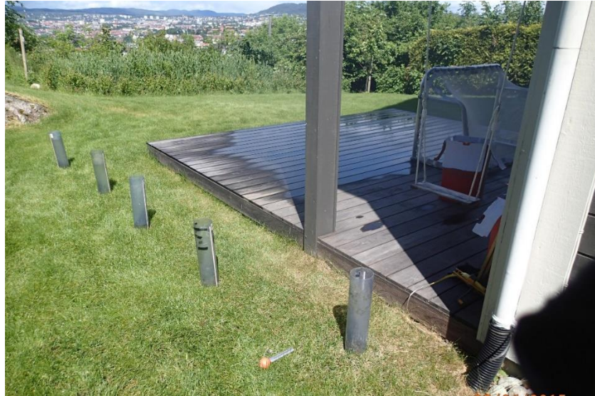
Figure 6.5 Set up for measuring saturated hydraulic conductivity with MPD.(photo: Mareike Becker)
