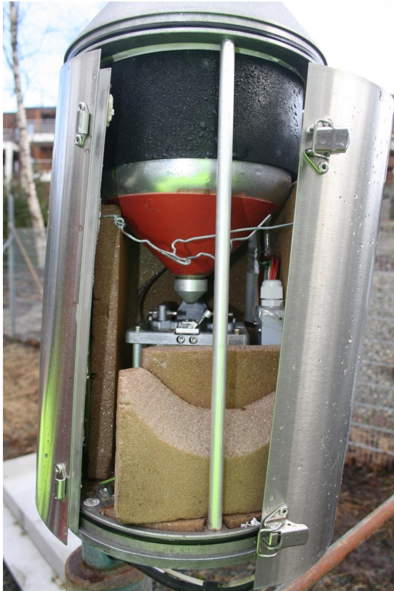
Figure 12 Inside of the Lambrecht gauge
