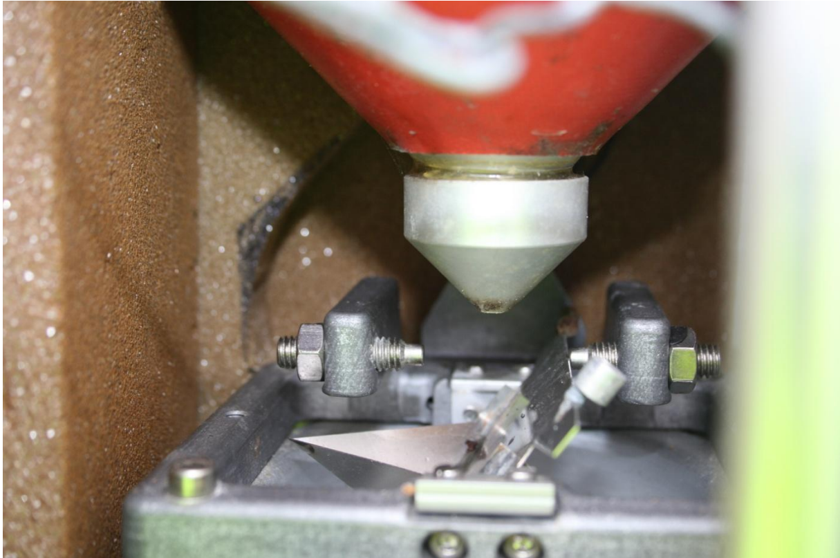
Figure 13 Presentation of triangulates pyramids inside the Lambrecht gauge
