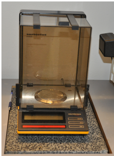
Figure 4.11: Balance Sartorius Analytic A200S
