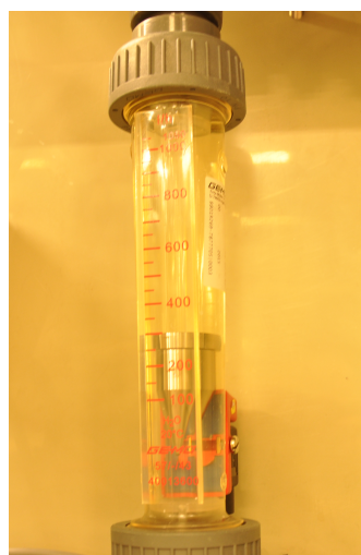
Figure 4.8: Details of the flowmeter
