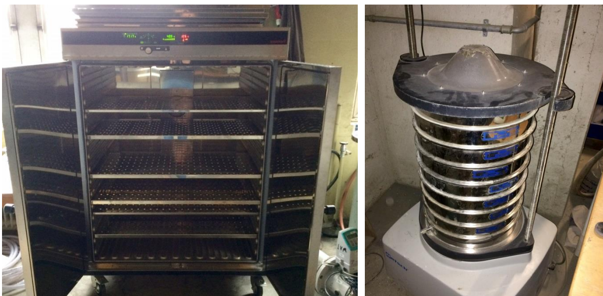
Figure 6-2 Heating oven to dry the gathered samples (left) and the siever machine (right)
