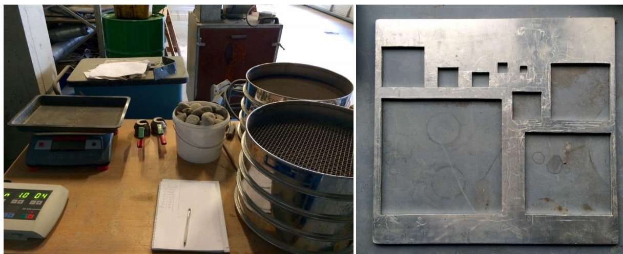
Figure 6-3 Scale with a few sieving particles (left) and a handmade Wentworth template (right) Particles larger than 64 mm were measured with a Wentworth template, which was made in the laboratory in 2010 (Figure 6-3, right). It helped to determine heavier pieces in the sediment samples, and sort of classes between 64 – 128 mm and 128 – 256 mm.
