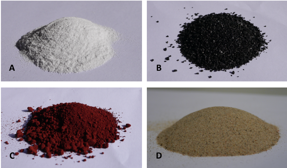
Figure 14 Other sorbents: A) Aluminum oxide, B) activated charcoal Norit®, C) Iron(III) oxide and D) sand
