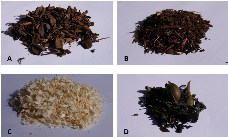
Figure 13 Biosorbents: A) Pine bark, B) Spruce-pine bark, C) sawdust and D) ascophyllum nodosum .
