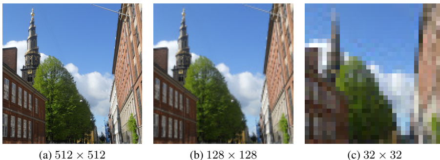
Figure 2.3 – Illustration of the impact of image sampling choices to a color image. Reducing spatial resolution will cause a pixel to cover a larger area and, consequently, smaller details in the scene are not captured.
