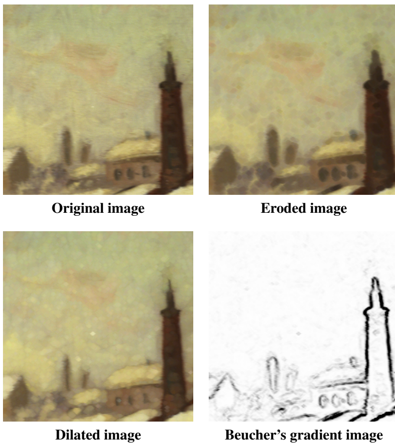
Figure 7.6 – Image FN1, eroded and dilated with disk SE of 2 pixel radius. CRA ordering relation is employed, embedding KLPD function and spectral references S_{Bk} and S_{Wh} . Beucher's gradient image is obtained using KLPD function.
