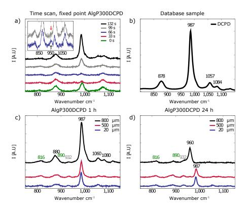
Figure 5: **a):** Raman spectra of an AlgP300DCPD sample from a single spot at 5 time points. The inset shows a close up of the 66 s and 99 s plots where a peak located at 955 cm<sup>-1</sup> is visible after 66 s (black arrow) and gone after 99 s (red arrow). **b):** Raman spectra of phase pure DCPD prepared in solution. **c)** and **d):** Raman spectra from a line scan of an AlgP300DCPD sample after 1 and 24 h respectively.
