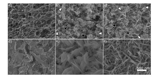
Figure 7: SEM-images of an AlgP300 sample gelled and mineralized in a 1 M CaCl<sub>2</sub> solution at pH 5. **a**), **b**) and **c**) are recorded from a sample incubated in the gelling solution for 1 h, while **d**), **e**) and **f**) are recorded from a sample incubated in the gelling solution for 24 h. Black arrowheads indicate to selected alginate/mineral nodules. White arrowheads indicate selected flaky plate like crystals. The scale bar applies to all of the images in this figure.
