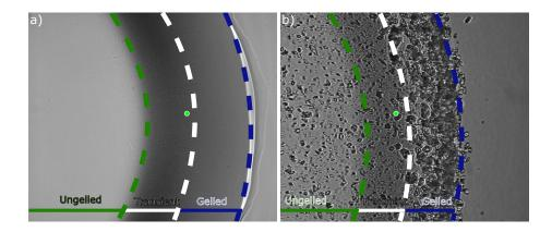
Figure 2: Phase contrast microscopy images showing an AlgP300 (**a**) and an AlgP300DCPD (**b**) sample during the gelling process. Three regions are marked in the images: the ungelled region shown in green, the transient zone shown in white, and a gelled region shown in blue. The marker indicates the approximate position of the CRM time scan. The frame width of the images is 845 µm.
