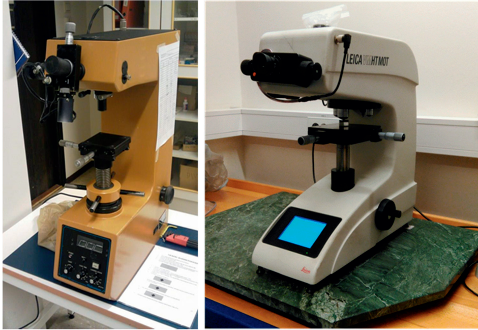
Figure 61. The Matsuzawa macro-hardness indenter (left) and the Leica VMHT MOT micro-hardness indenter (right).
