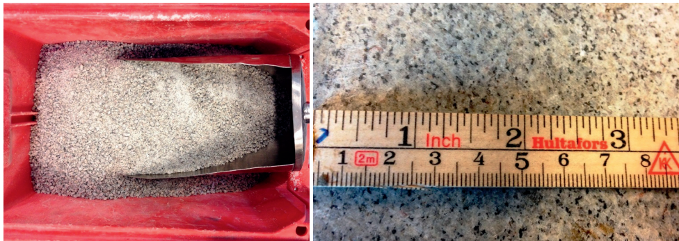
Figure 51. The Iddefjord granite. A crushed rock sample (left) and intact rock (right).
