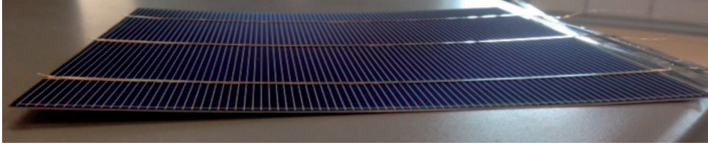
Fig. 2. Bending induced in a silicon wafer through mismatch in thermal expansion coefficients of the Cu-ribbon and wafer upon cooling. (Adapted from [33].)
