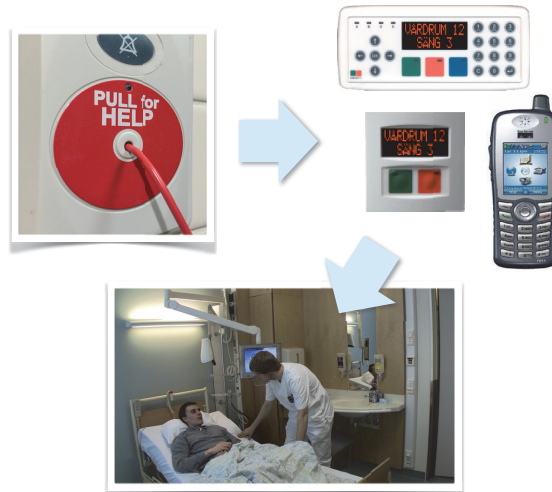
Figure 1.1: Illustration of the general principles of a nurse call system. The patient pulls a draw-string to communicate the need of assistance. Nurses get notified through a receiving device and respond by visiting the calling patient. (Left upper photo by Tony Webster, right upper photos form Mathiesen (2005))
