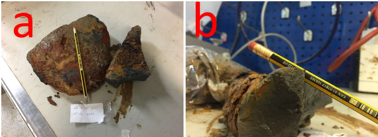
Figure 24: Rock sample from the area N of S11 where some type of venting is suspected. a) staining on fractures b) py grains on the rim towards the fracture plane. Photo: NTNU MarMine / Kurt Aasly
