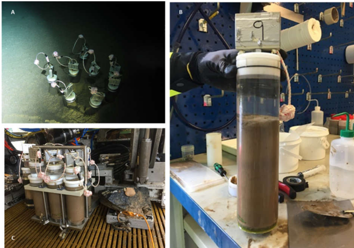
Figure 34. Push-cores in the sediment (A), the rack of push-cores after recovery in the front of the ROV (B) and a push-core in the lab ready to be processed (C).
