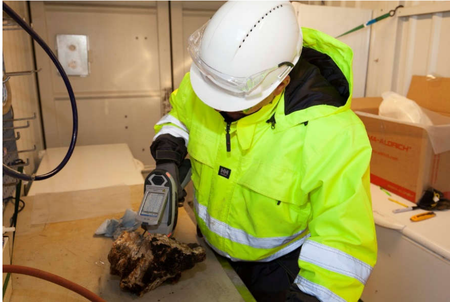
Figure 12. The handheld XRF was used to get a rough indication of the element content of the sampled rock samples.
