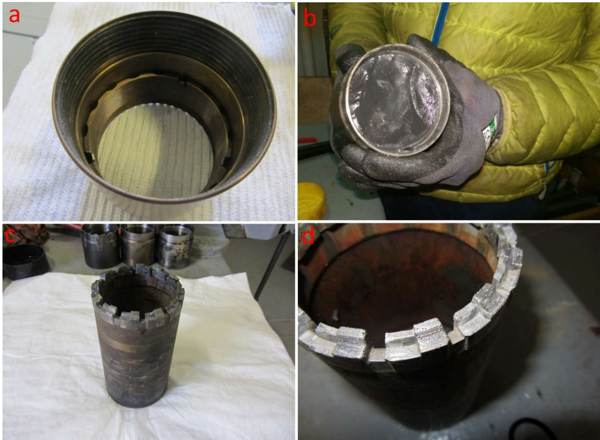
Figure 38: a) Modified hard rock core lifter; b) Core retained in core lifter case; c) 350C Series 14 thin kerf core bit; d) Core bit impregnated diamond cutting surface
