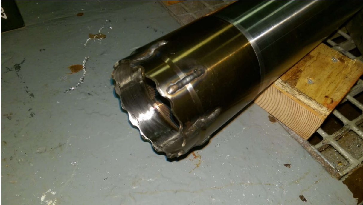
Figure 37: Modified core lifter case for soft sample.
