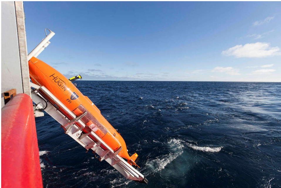
Figure 4: Hugin in the stinger, while being deployed.
