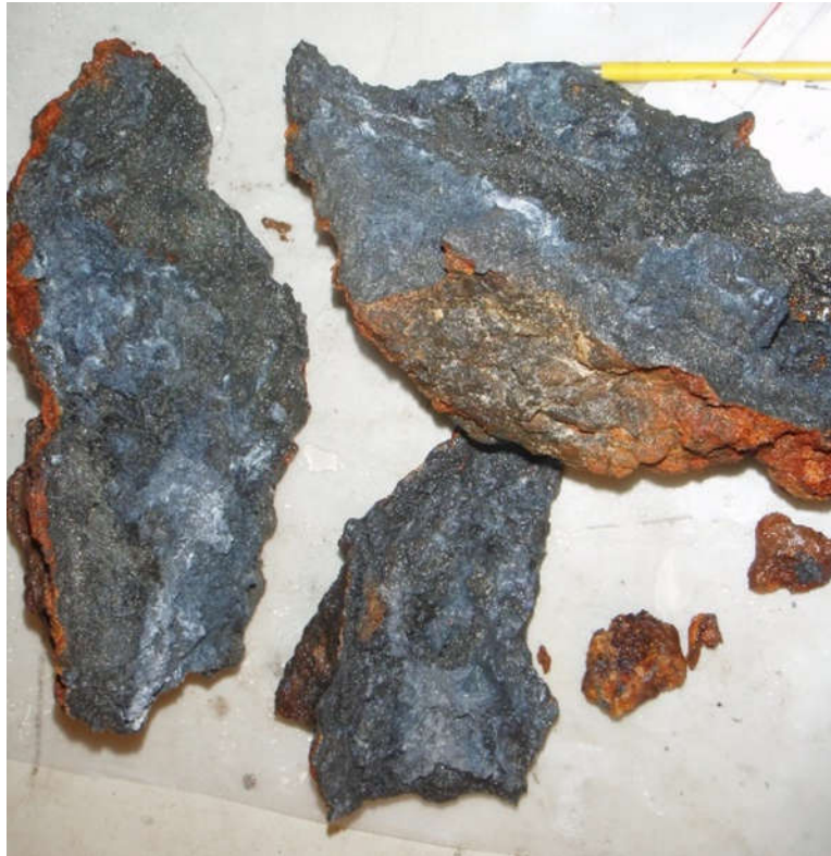
Figure 21: Samples from LC. Chimney fragments with visible fluid channels with mineralization. Photo: NTNU MarMine / Kurt Aasly
