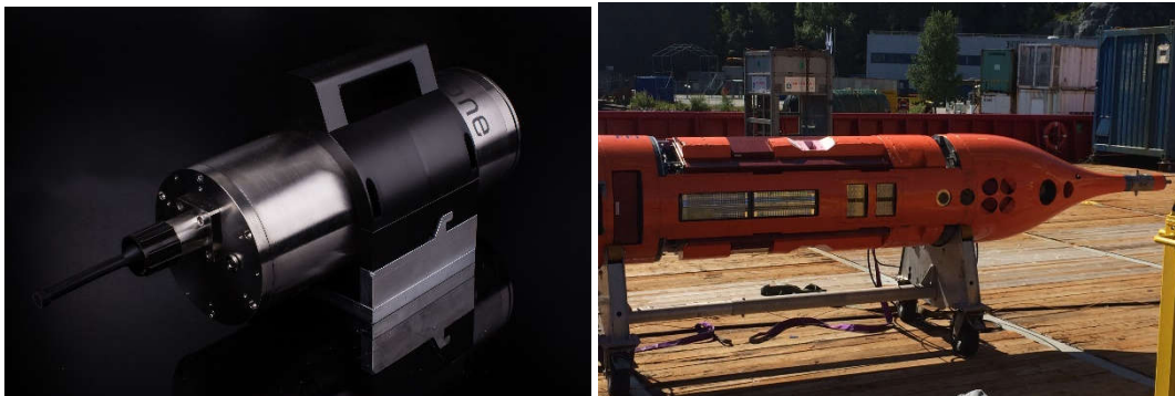
Figure 8. The UHI sensor and the AUV with the sensor mounted. The AUV has a roll angle of 90° in the picture.
