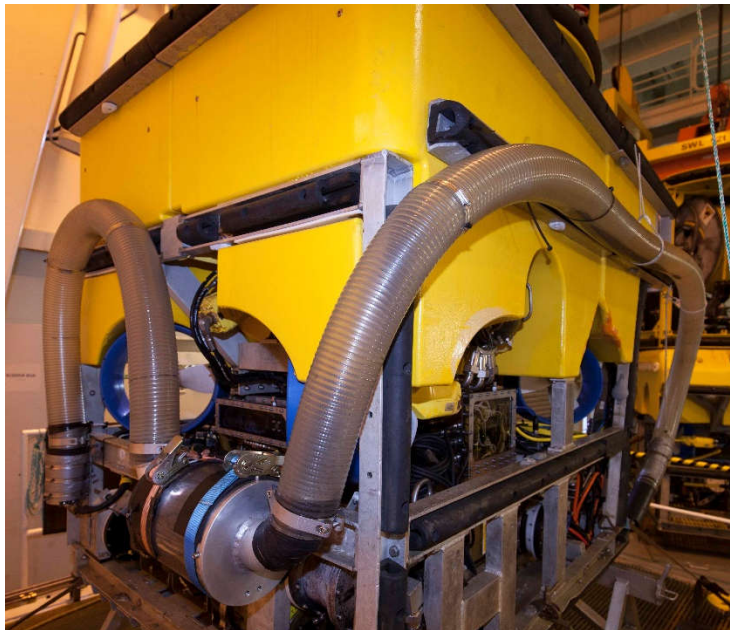
Figure 15: Suction sampler mounted on the XLR02 ROV. Photo: NTNU MarMine / Lars Ivar Tumyr.
