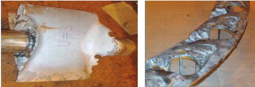
Figure 12. Sediment erosion damage in GV and facing plates. Adapted from Alam [6]
