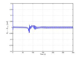
Fig. 9. The head angle tracking error.
