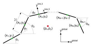
Fig. 1. Kinematic parameters of the snake robot.
