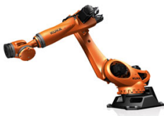
(a) The KR 270 R2700 ultra Industrial Robot, produced by KUKA.
