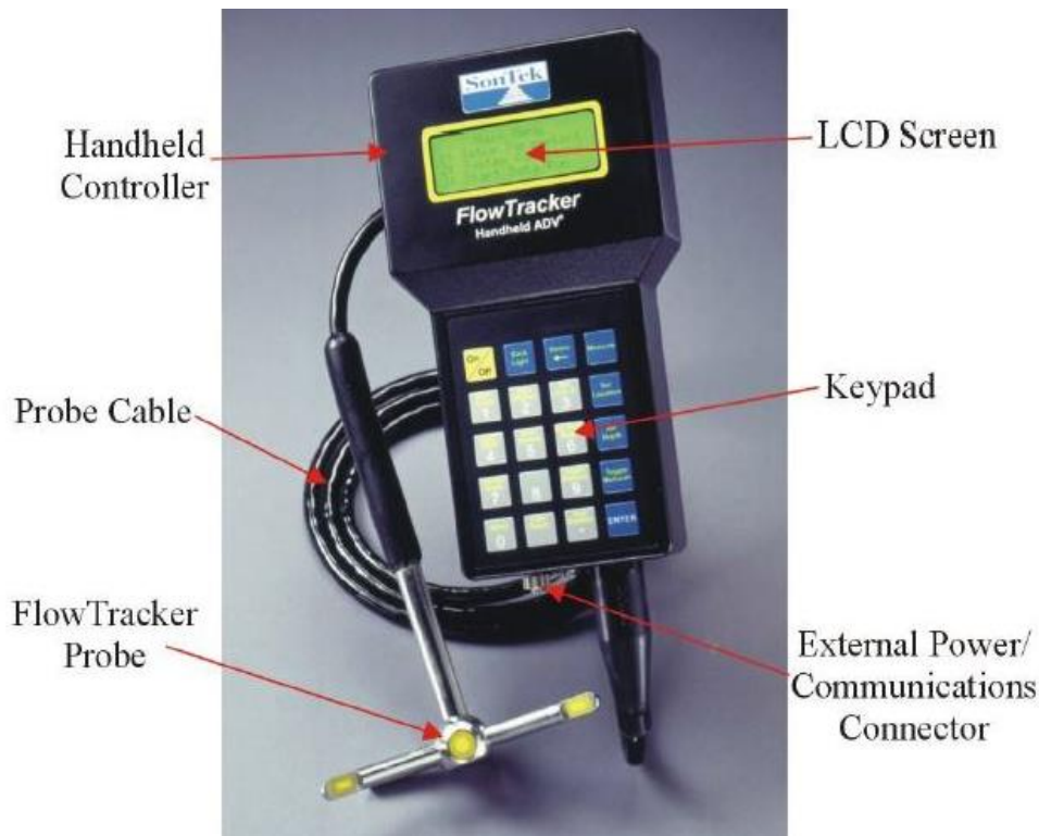
Figure 3-2. Major components of Flow Tracker. ( www.sontek.com , 2007)
