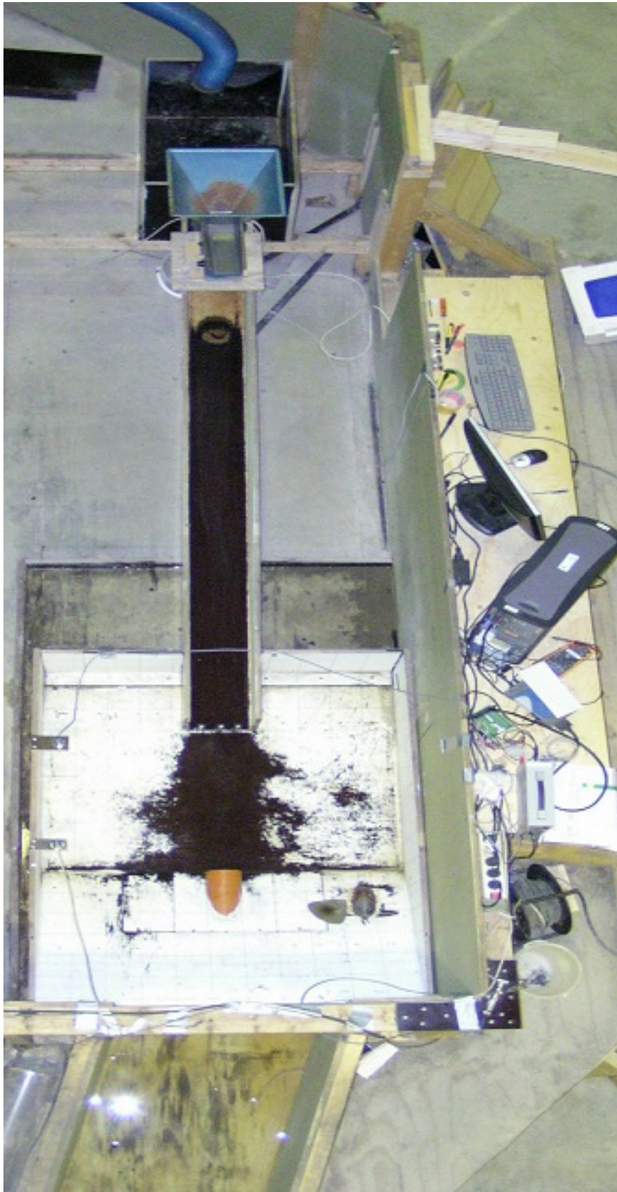
Figure 3.3 A Picture of the whole culvert model
