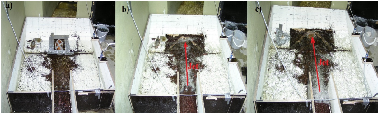
Figure 4.9 Flow conditions in the expansion section for system operating with a) only reserve barrel, b) multibarrel and c) only main culvert.
