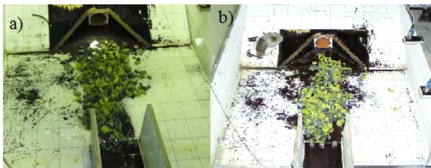
Figure 5.3 Sediment deposition pattern in a) single barrel and b) multibarrel system.
