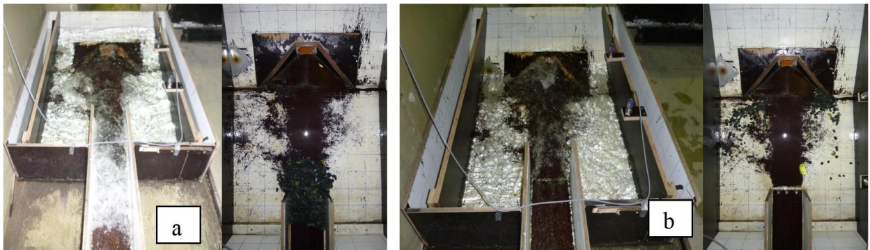
Figure 4-35 Hydraulics and deposition pattern with wing wall inlet at 10 l/s using sediment amount of: a) 7 kg, b) 5 kg
