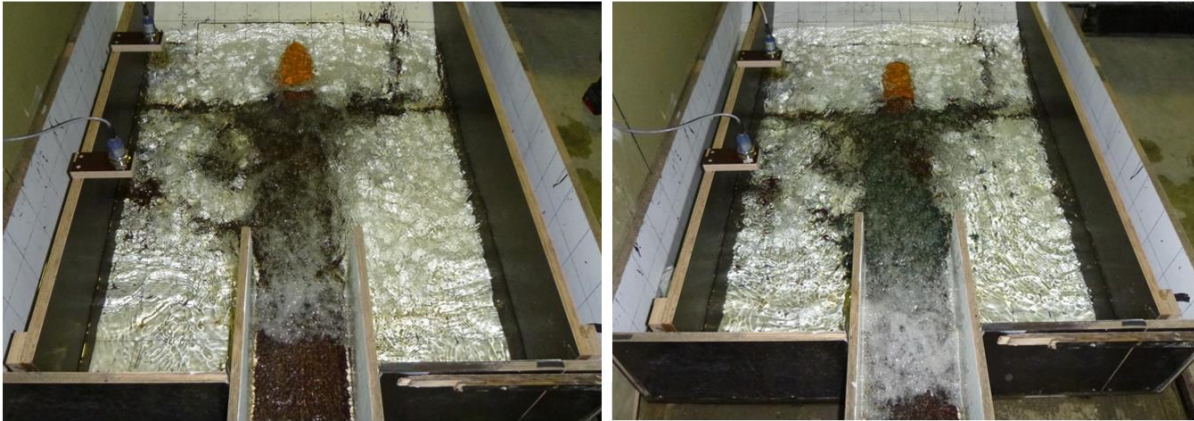
Figure 4-33 Changes on the water depth at 8 l/s with 7 kg amount of sediment
