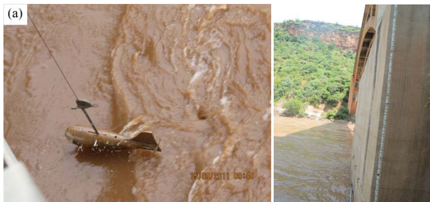
Figure 3.5 (a) suspended sediment sampling at Burie bridge, (b) stream flow gauging and sediment sampling station at Kessie Bridge (Photo by: Dr. Kiflom Belete)
