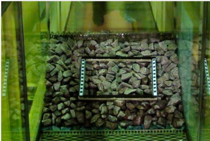
Figure 6.2 Packing factor for yellow stones
