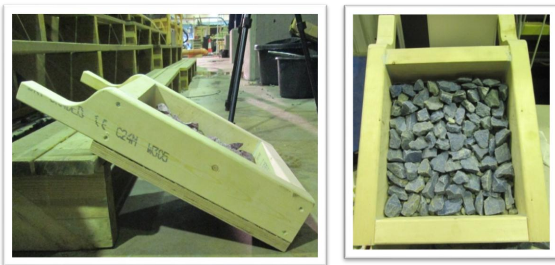
Figure 6.1 Experimental setup for the angle of repose measurement
