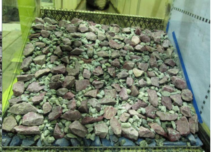
Figure 6.16 Scaled Model of the prototype dam
