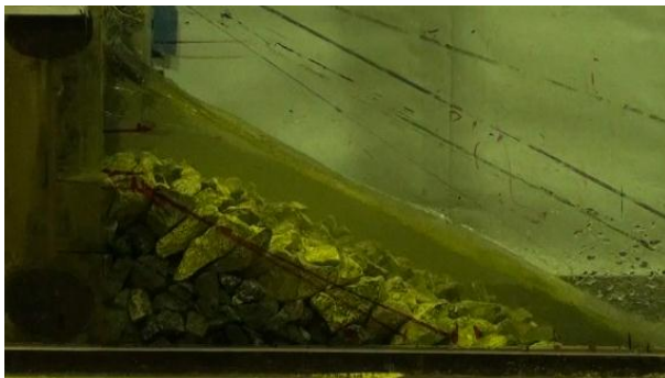
Figure 6.20 71 degree orientation for the yellow stones
