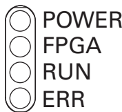
Figure 9. NI 9144 Chassis LEDs
