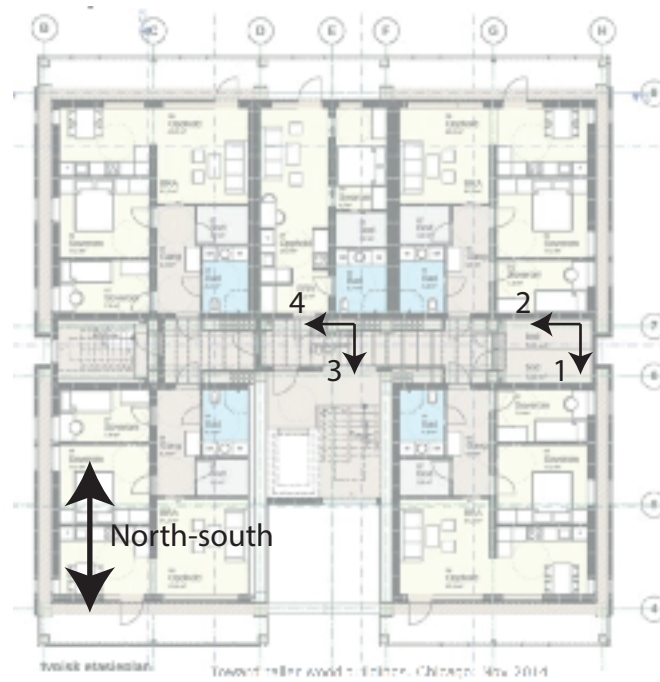
Figure 1: Plan of a typical storey, showing the location and direction of accelerometers and their channel numbers
