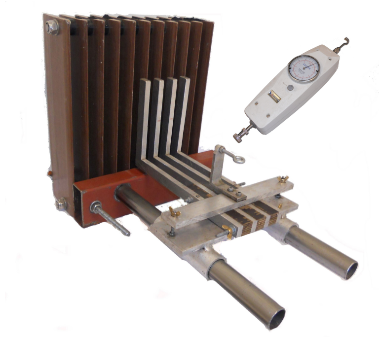
Figure 2.7: Pulling Equipment for Evaluation of Trash Rack Adhesion («PEETRA»)
