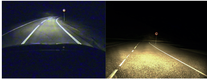
Fig. 2. Example of the driver's visual impression on the closed-circuit test track (left) and in the driving simulator (right).
