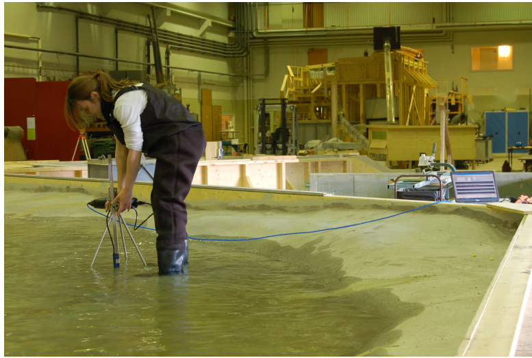
Figure 3.5.: Positioning the Vectrino Velocimeter above a measuring point, photo: N. Olsen
