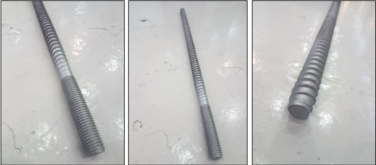
Figure 40: Threaded rod side with M20 (left) and the threads designed for wood-insertion (right)
