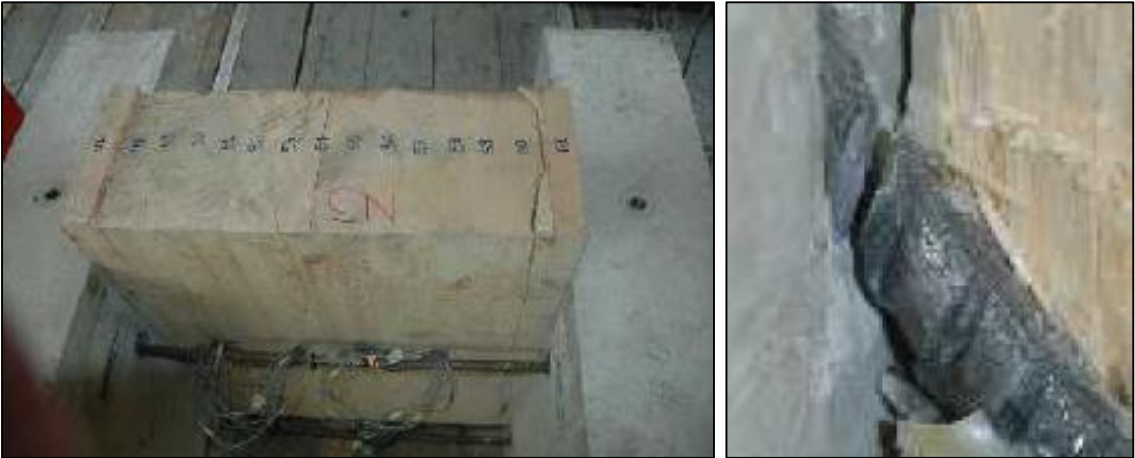
Figure 30: Failure modes subjected to static load in grooved connections (left) and x-connectors (right) [36]
