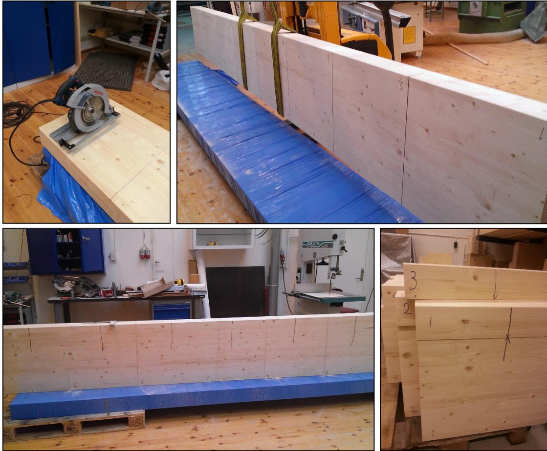
Figure 36: Cutting of specimens and numbering according to placement in the beam, 90°
