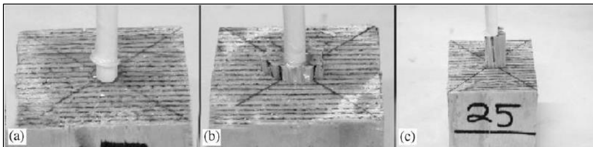
Figure 18: Failure modes in stress-rate-effect study (a) 0.5 mm, (b) 2 mm and (c) 4 mm glue-line thickness for LVL
