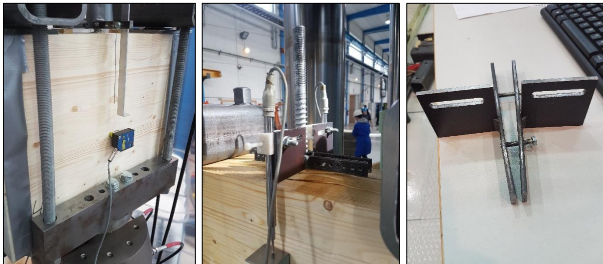
Figure 45: LVDT, laser (left) and push rod (middle), support to the rod (right)
