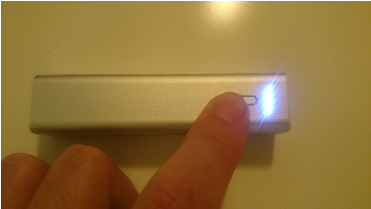
Figure 3.5: 2600mAh lithium ion battery pack with four blue lights indication remaining charge when button is pressed.
