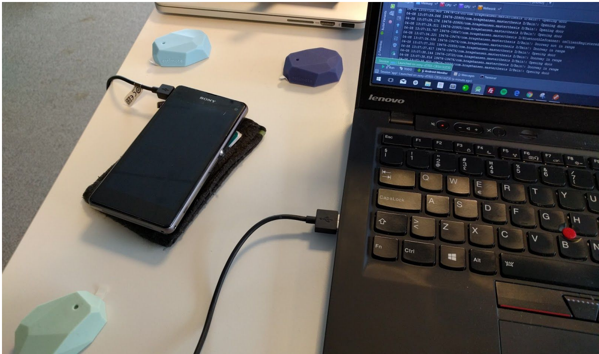
Figure 3.7: A Windows 10 laptop running Android Studio 1.5.1 while connected to a Xperia Z1 Compact Three. Three estimate beacons are being ranged. The computer is showing debug data displaying the beacons reported distances to the phone using the Estimote SDK for ranging based on RSSI signal strength.
