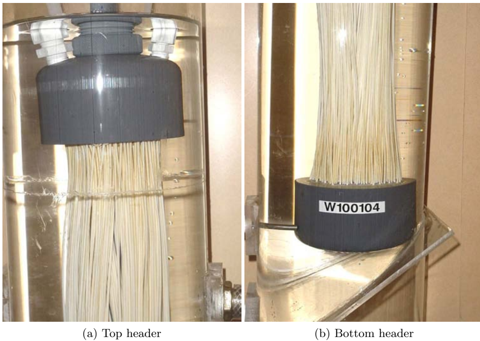
Figure E.1: Module headers with fibre bundle immersed in distilled water. Inclined plate settler visible in the bottom.
