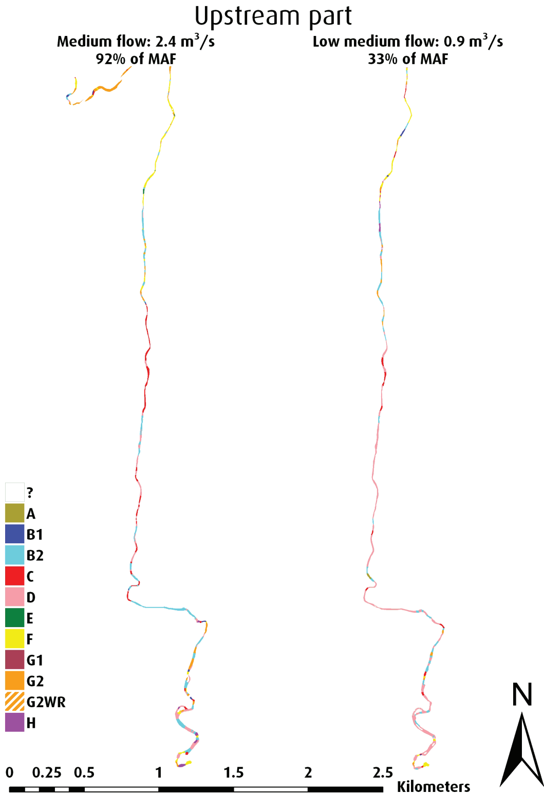
Figure 2.9: HMU maps at 0.8 (33% of MAF) and 2.4 m 3 /s (92% of MAF) of Ingdalselva, upstream part
