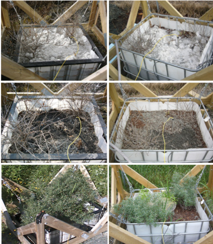
Figure 3.6: Field pictures from the snowmelt study in April 2006. The two top pictures were taken just after snow was applied to the bioretention boxes. The middle row of pictures shows the grey layer of sediments and pollutants on top of the mulch layer after the experiments. The bottom pictures show the bioretention boxes 2 months later with vegetation fully recovered.
