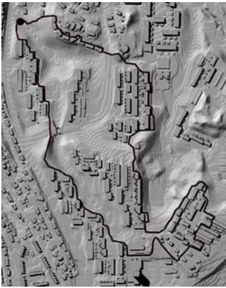
452 Figure 1. Digital elevation map (DEM) of the watershed with buildings included in the model, and 453 grid cells of 1 by 1 meter. Watershed outlet at location marked with a dot in top left corner. 454
