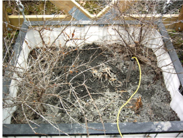
Figure 5.3: The top mulch layer on bioretention box 1 after the snowmelt studies in April 2006.
