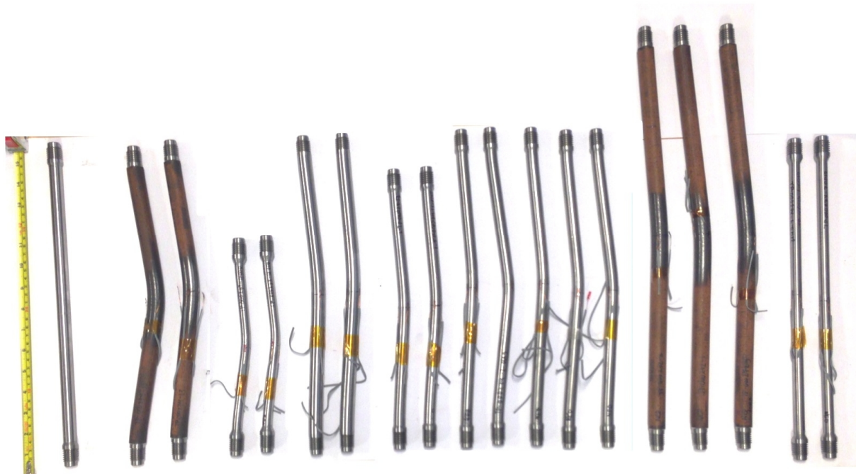
Figure 6.3: Buckled test parts sorted by slenderness-ratio from left; lowest to highest.
