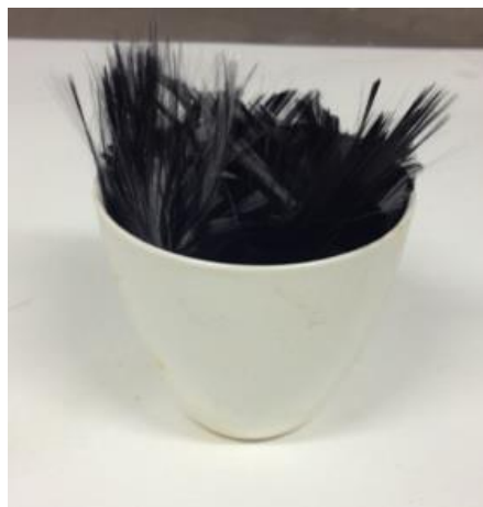
Figure 16 Fibers left after the epoxy evaporated
