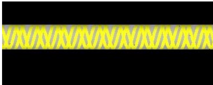
Figure 14 3 over 1 pattern used to wind the tubes
