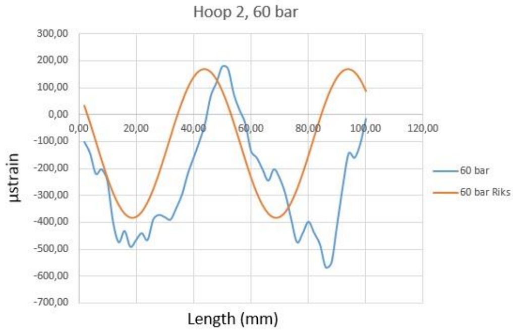
Figure A10 Comparing strain at 60 bar in hoop 2
