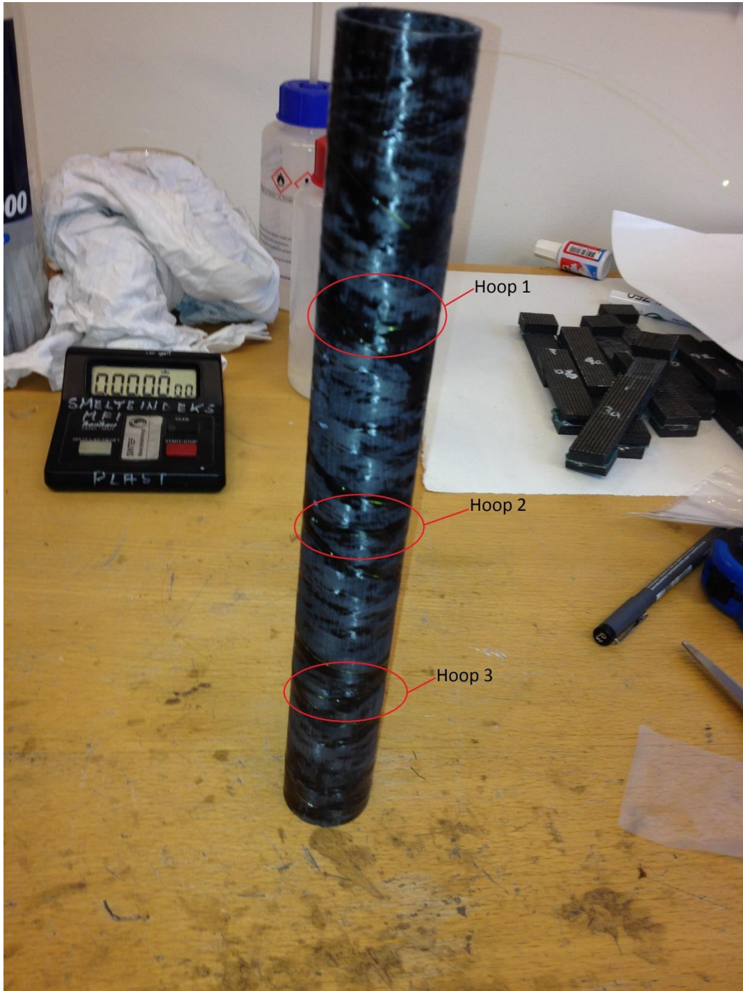
Figure 20 Optical fibers attached to the tube in hoops
