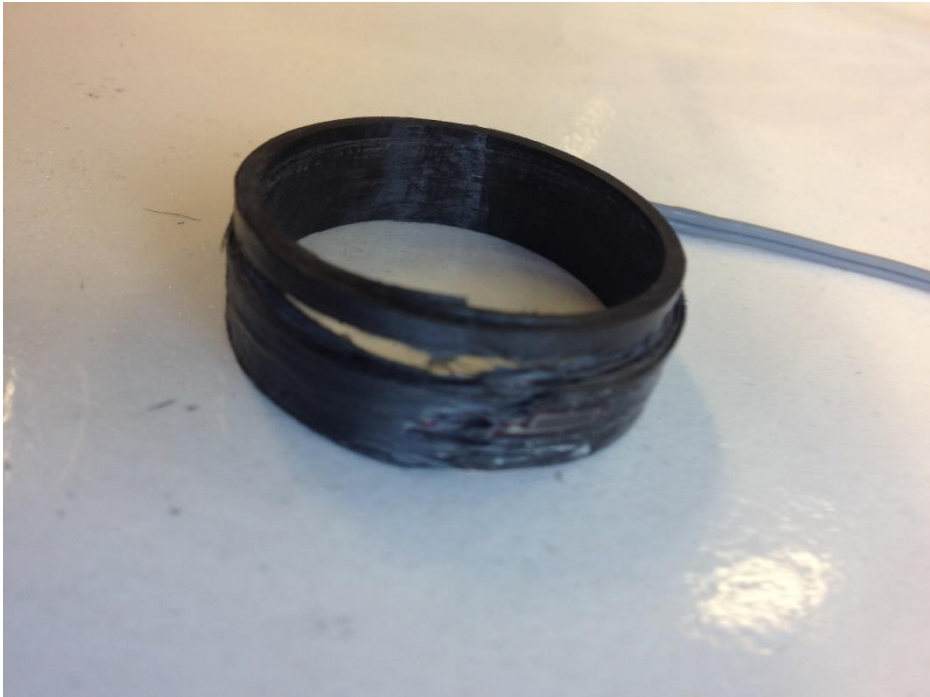
Figure 31 Failure of the ring tested with the split disc method
