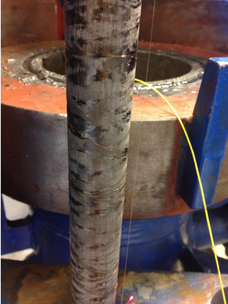
Figure 25 Damaged optical fibers are detected with a laser glowing red at the damaged area
