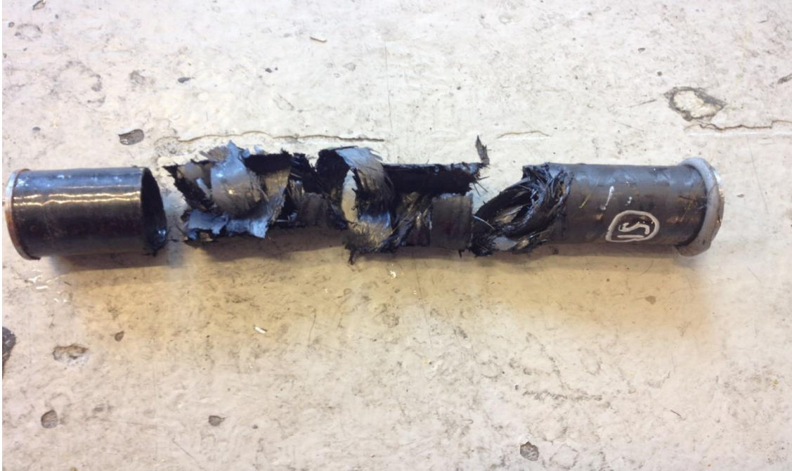
Figure 40 Failed tube after external pressure test
