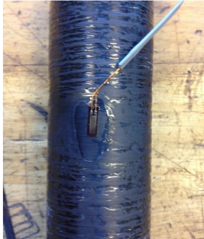
Figure 26 Strain gauge attached to the tube perpendicular to the fiber direction
