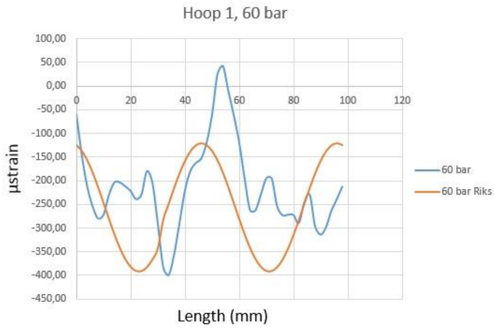
Figure A3 Comparing strain at 60 bar in hoop 1
