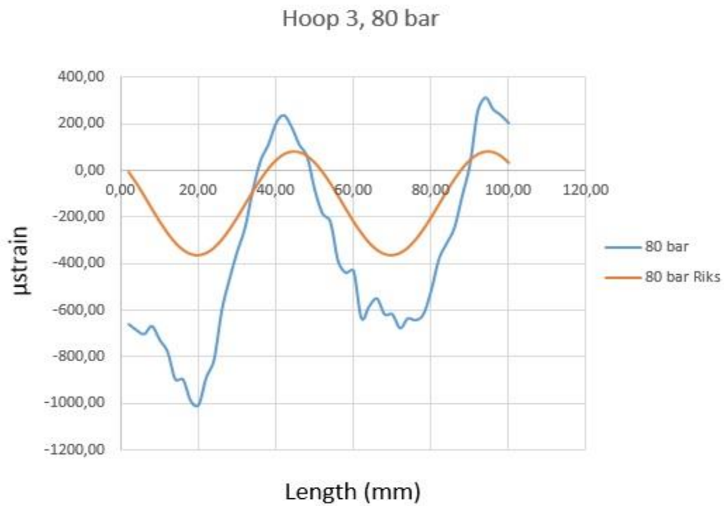
Figure A18 Comparing strain at 80 bar in hoop 3
