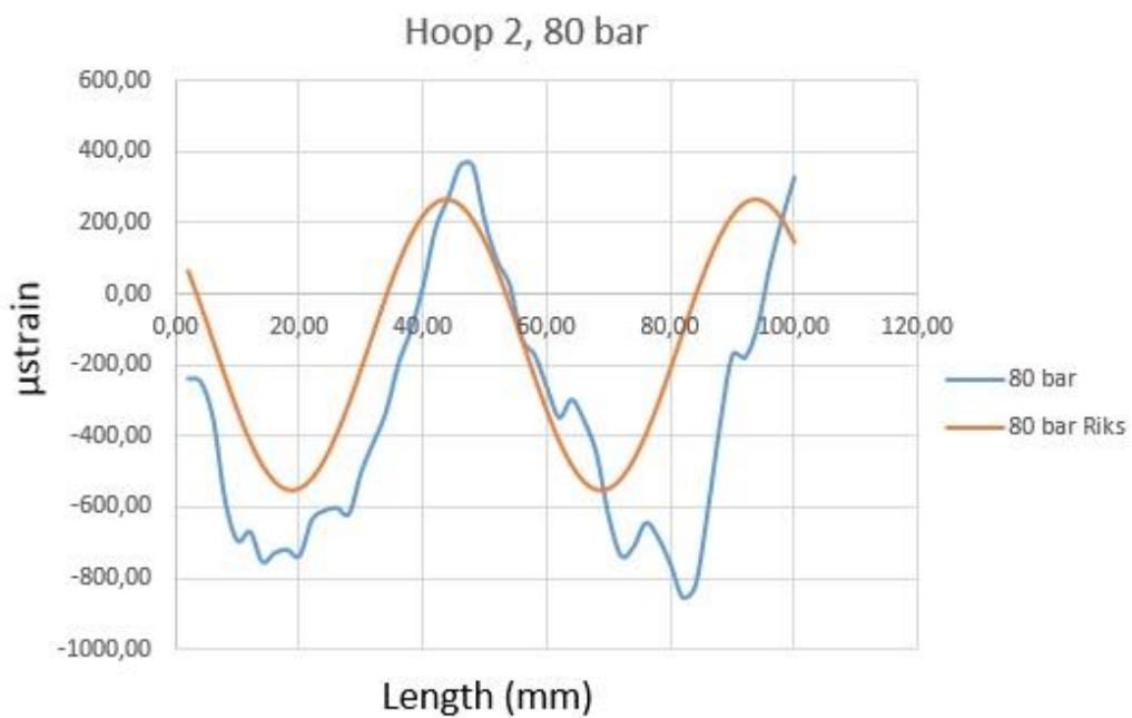
Figure A11 Comparing strain at 80 bar in hoop 2
