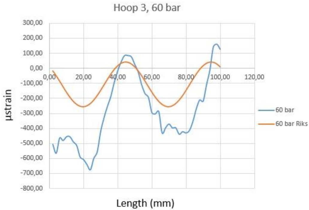
Figure A17 Comparing strain at 60 bar in hoop 3
