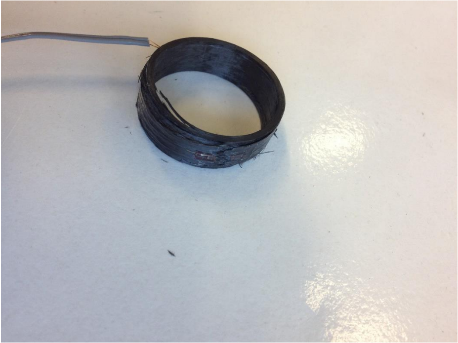
Figure 32 The ring tested using the split disc method failed at the location of the strain gauge
