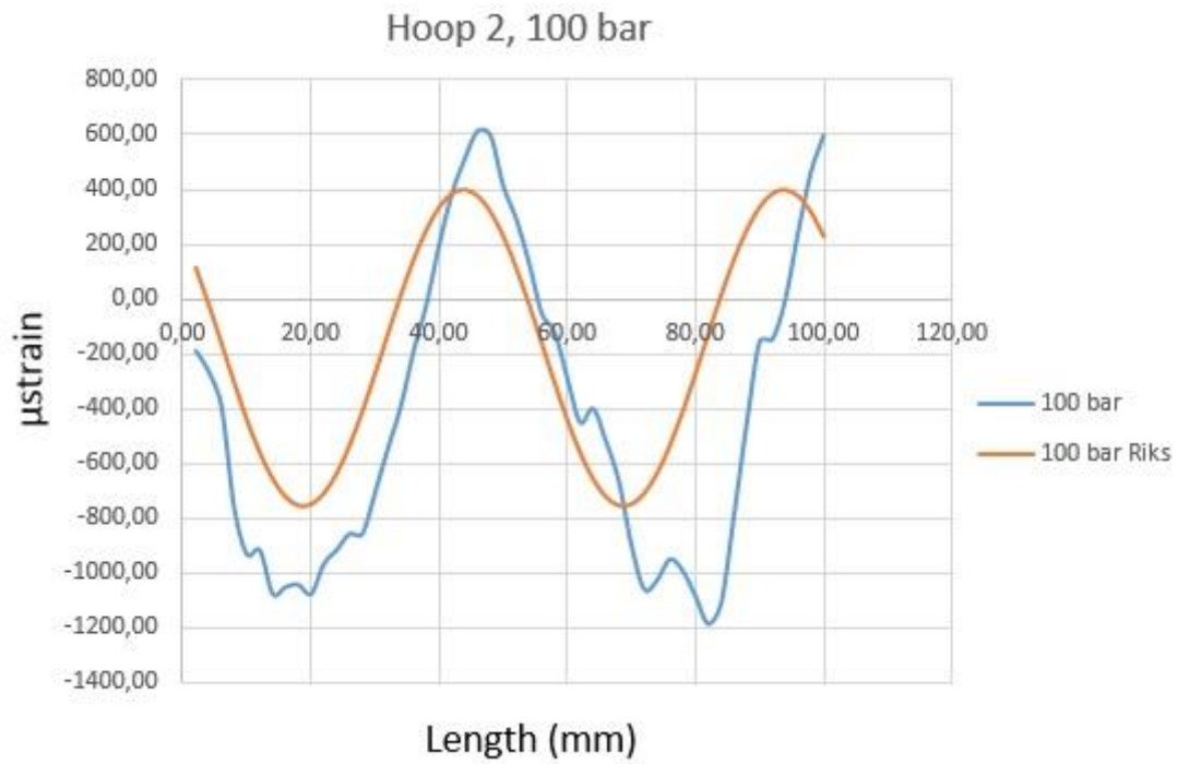
Figure A12 Comparing strain at 100 bar in hoop 2
