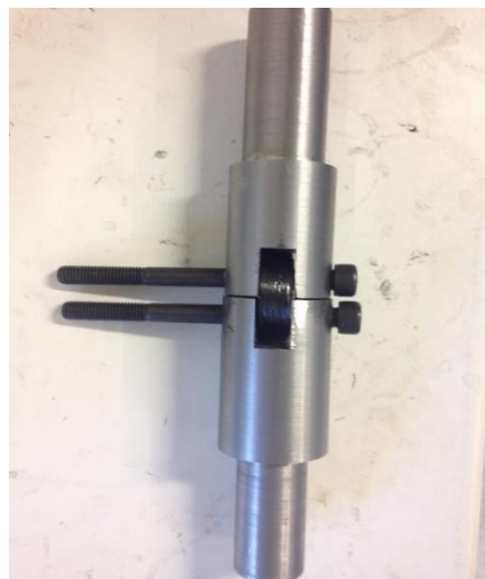
Figure 28 Split disc fixture with the split disc and test piece installed
