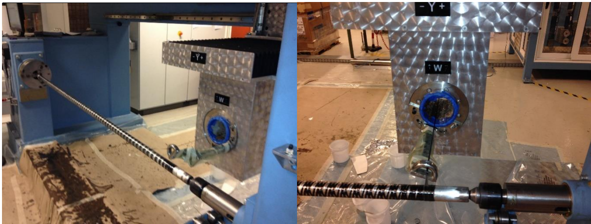
Figure 13 Filament winding process with the rotating mandrel and the eye controlling the angle of the fibers
