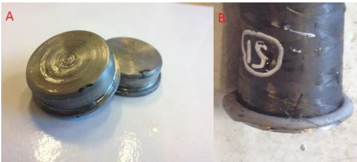
Figure 24 A shows the end caps before they are mounted on the tube, while B shows an end cap fitted into the tube and sealed with “stickytape”
