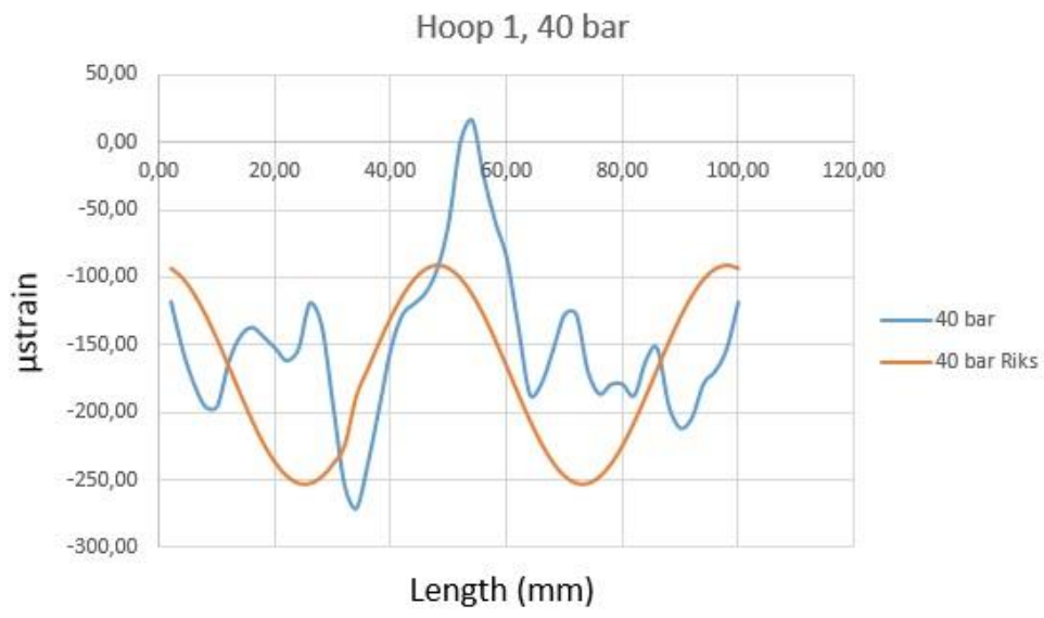
Figure A2 Comparing strain at 40 bar in hoop 1
