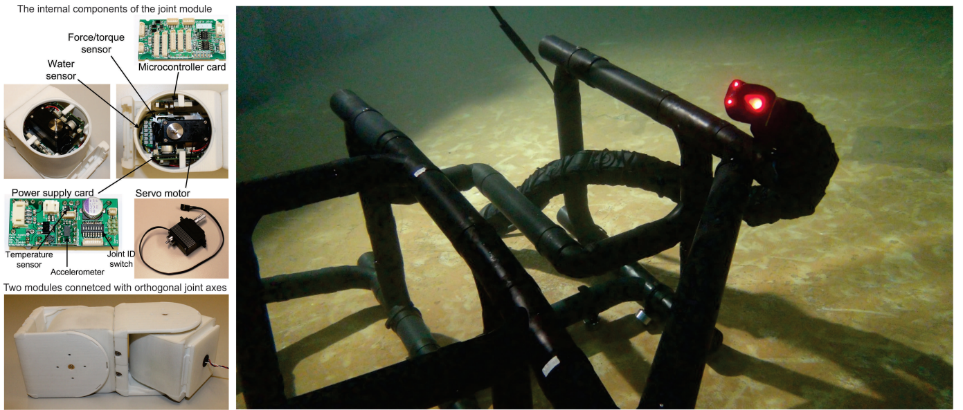
Fig. 5. The underwater snake robot Mamba implemented at NTNU to support our group's research activity about both ground and underwater snake robot locomotion.
