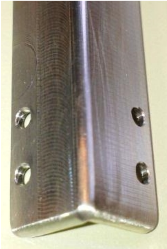
Figure 94: Left side milled from top, right side milled from side
